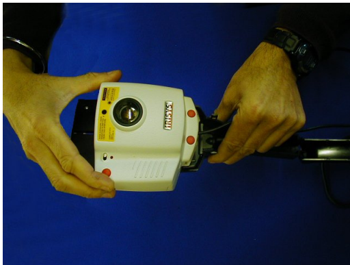
17) Push the imager down onto the pegs, so that it locks down into position.
