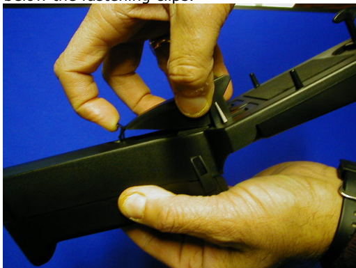
3) Un-clip the cable connector cover.
