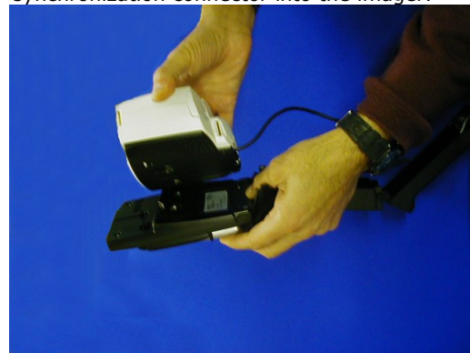
16) Line up the holes on the back of the imager with the pegs on the handle.
