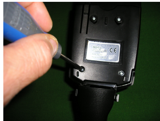
2) Remove the Pocket PC hooks by unscrewing the two screws from the front of the handle
