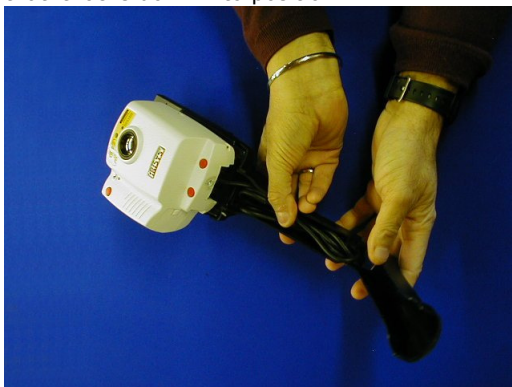
19) Push the coiled up cable into the handle grip.
