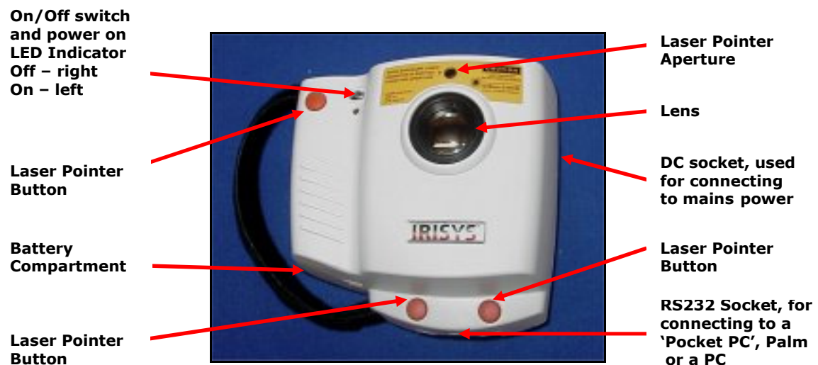
Figure 4: The IRISYS IRI 1011 Universal Thermal Imager.
