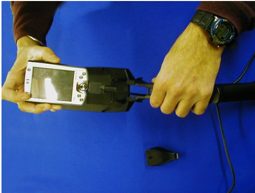
7) Pull the cable through the handle so that the 'Pocket PC' can sit on the back of the handle.
