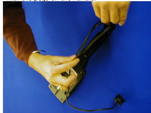
18) Coil up the serial synchronization cable, so that it will fit into the handle grip.
