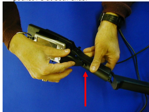
12c) The bottom end of the cable cover is then slotted into the handle.
