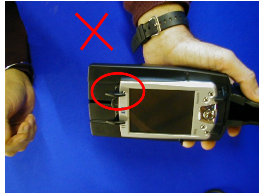
10) Example: with the clip around the wrong way it may cover the Pocket PC power button.
