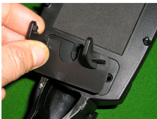
3) Turn the handle over and remove the Pocket PC hooks and replace with the Palm Hooks.
