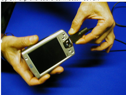
5) Connect the serial synchronization cable into the 'Pocket PC'.
