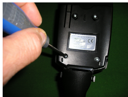
4) Fasten the Palm hooks by screwing back the two screws at the front of the handle.
