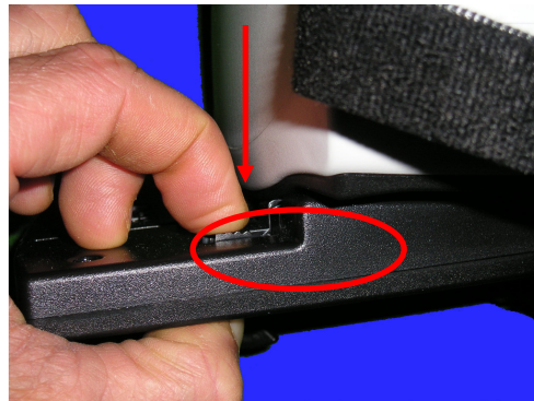
2) Press the release lever down.
