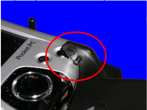
12a) Note the locators near the bottom of pocket PC at both ends.
