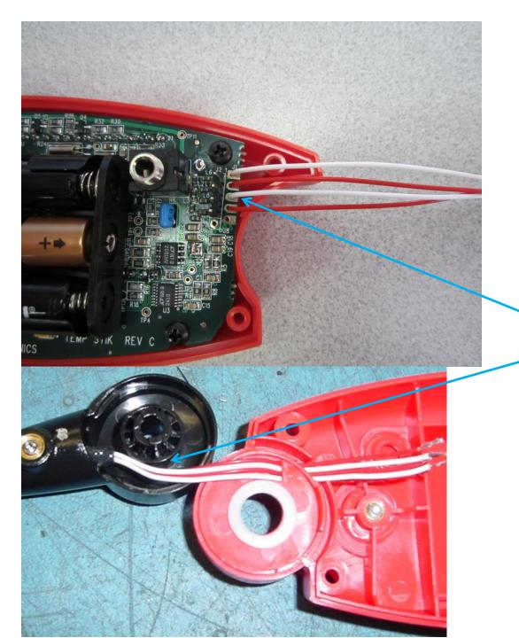
Verify that the wires have not broken off the PCB or broken or been pinched in the elbow.
