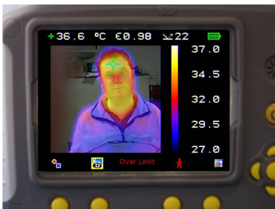
Figure 1 Imager fusion showing over limit alarm
