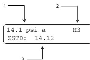
1. Pressure reading, units and mode of the active Hi RPT range.
