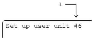
1. Entry field to select which unit position (1 - 6) of the UNIT function key menu is to be changed.
