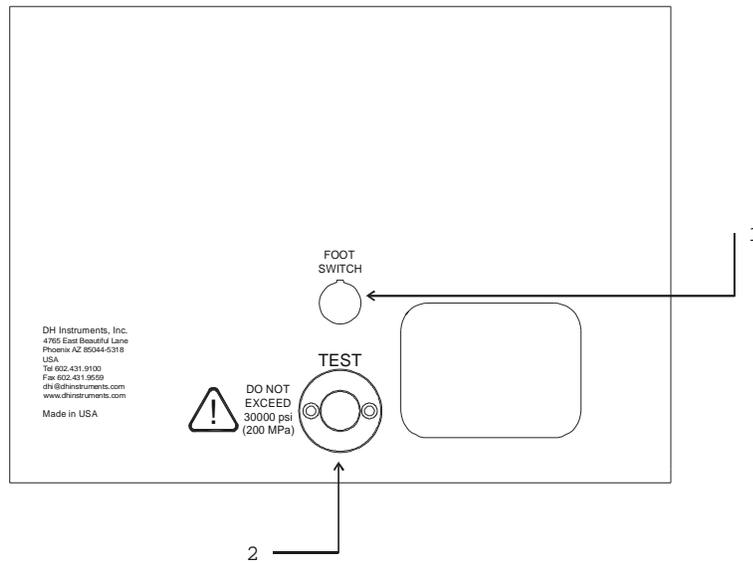
1. Foot switch (Remote [ENTER]) cable connection
