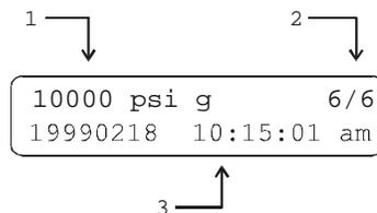
1. Full scale of the Sequence DUT with pressure unit of measure and measurement mode.
