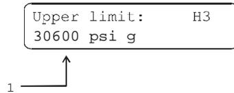
1. Edit field to view current upper limit value and modify if desired. The value is always in the current unit of measure.
