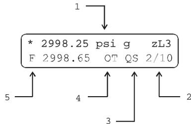
1. Conventional RPM3 main run screen indicating current measured pressure (see Section 3.1.2).
