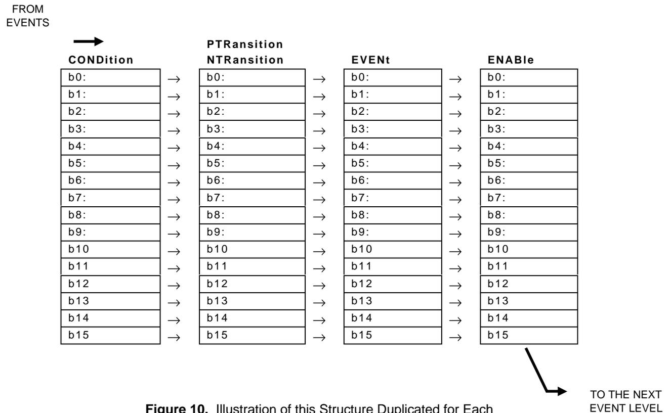
**Figure 10.** Illustration of this Structure Duplicated for Each of the OPERation, INSTRument, and ISUMmary Registers
