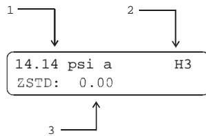
1. Pressure reading, units and mode of the active RPT range.
