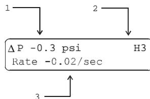
1. Net change in pressure over the leak check time period.
