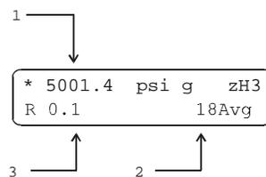
1. Instantaneous pressure values at RPM3s normal integration rate.
