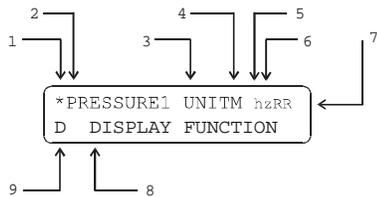
1. **<◀▶>** *Ready/Not Ready* indication, **<◀▶>** when *Ready*, **<↑>** or **<↓>** indicating direction of measured pressure evolution when *Not Ready* (see Section 3.1.5).
