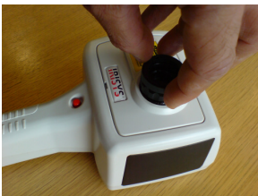
Figure 3. Filter being screwed into place.
