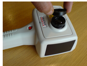
Figure 2. Filter being fitted.
