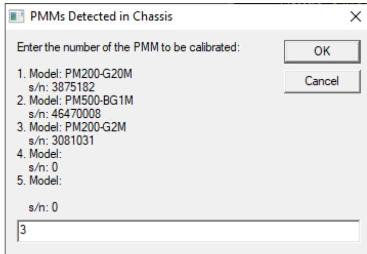
After the PMM selection is made then COMPASS progresses through the steps of the Test Definition. At the end of the first pressure cycle the data is automatically evaluated using a linear regression and new coefficients are determined and written to the PMM. The As Left verification cycle is then automatically started.
