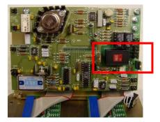
10. Use the hooked end of the insert removal tool to move the switch to the appropriate voltage setting (up for 115V down for 230V).
