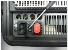
3. To set the heater switch, you will need to disassemble part of the 9009 to gain access to the heater switch. Now, close case securely and flip the 9009 over to gain access to feet on the bottom of the case. Remove the bottom (4) screws that are installed in the feet. These screws are sealed with silicone to prevent moisture entry.
