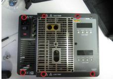
6. Turn over the instrument. Remove the 4 screws shown below.
