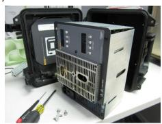
5. Set the case to the side. Put the instrument upright and remove the 6 screws shown below.
