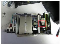
9. Use a flashlight to locate the switch. There is a black switch housing with a red switch under a voltage regulator.
